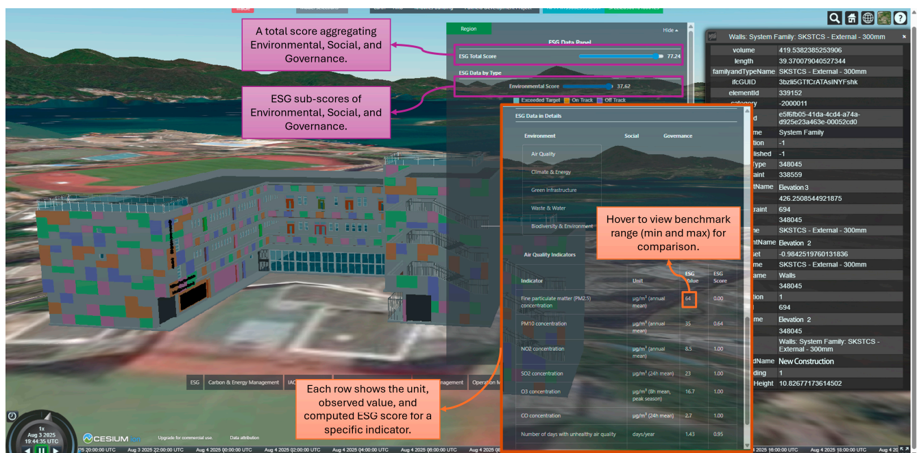
Figure 10. Web-based 3D visualization platform displaying ESG indicator results, building semantics, and environmental sensor integration in Cesium (The purple boxes highlight the total ESG score and its sub-scores and the orange boxes highlight detailed information for individual ESG indicators).
